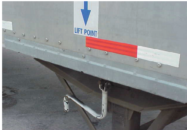
Fig. 4.6 Incorrect lift point
