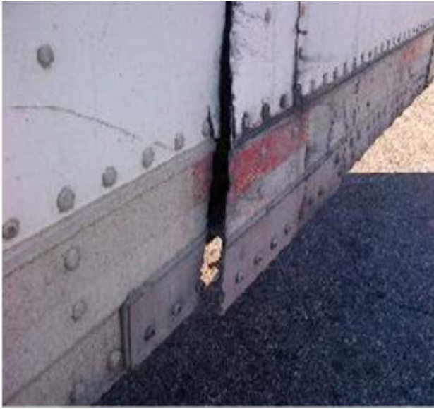
Fig. 2.4 Bottom rail break
