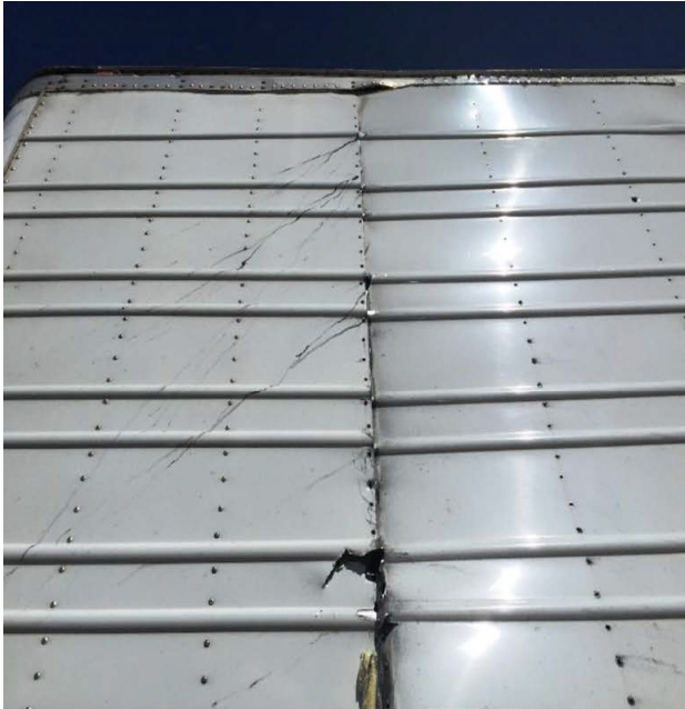
Fig. 2.31 Side panel securement defect
