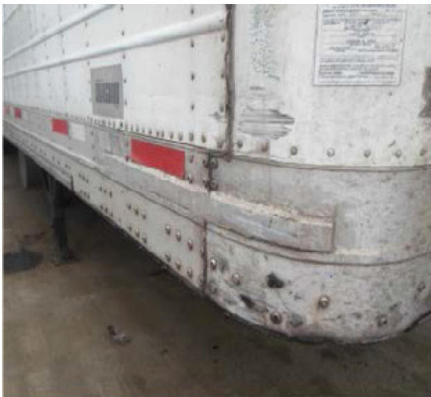
Fig. 2.14 Improper repair—welded patch
