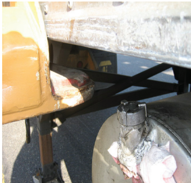
Fig. 8.2 Fuel tank damaged as a result of insufficient clearance
