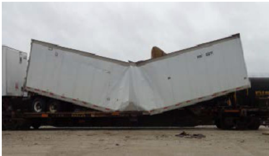
Fig. 2.1 Complete trailer failure
