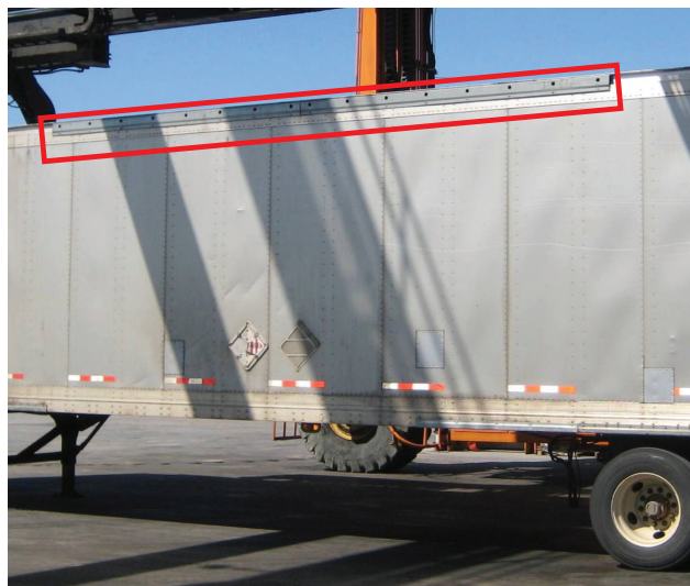
Fig. 5.1 Top rail protector—trailers longer than 40 ft
