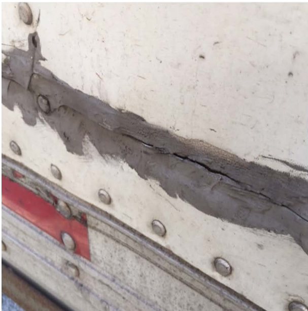
Fig. 2.27 Side panel breaks/cracks
